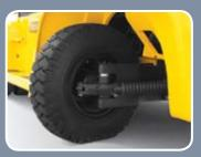
Fully hydrostatic power steering A hydraulic steering system always guarantees smooth and flexible steering, preventing overrun and kick-back.
