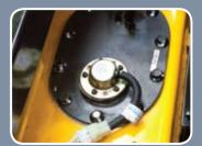
Fuel tank safety valve Integrated safety check valve shuts off fuel supply in the unlikely condition of a truck overturn.
