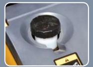
Brake fluid reservoir Highly visible, easily accessible reservoir makes for quicker daily inspections.
