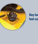
Key-locking fuel cap with air vent
