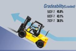
Travel speed(Unloaded) 50DF-7 22.8km/h 60DF-7 22.7km/h 70DF-7 22.7km/h
